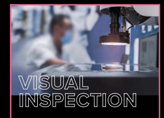
High-resolution cameras capture detailed images of machines and products in the manufacturing process. These images are then analysed by image processing algorithms, based on artificial intelligence (AI) and machine learning (ML), to detect the smallest errors or deviations with extreme precision. This data-driven approach, hosted on a cloud platform, provides real-time insights and ensures accurate quality control.
